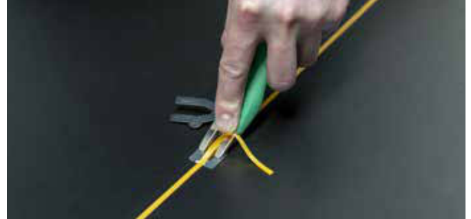
Simple reworking of welding seams with the Leister trimming knife.
